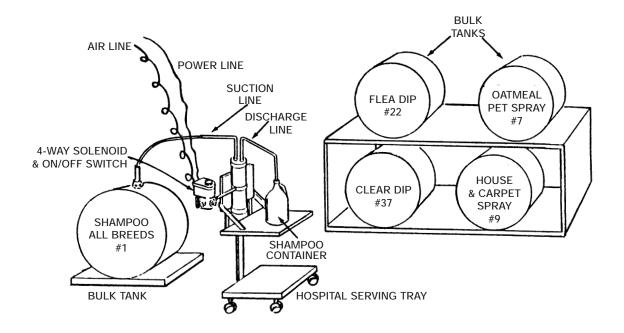
A national pet care products manufacturer required a method to increase productivity and safety in their filing process. Pet care liquids, such as shampoo and flea dip, have different viscosities and are sold in a variety of different size containers. The Plast-O-Matic Series VPA Metering Pump was selected not only for its accuracy of repeatability of 1/2 of 1%, but also for its ability to be adjusted down to 20% of the total pump volume, thereby
