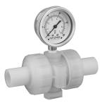
Unique in-line design eliminates "dead leg' that can harbor bacterial growth and contamination. Unpigmented thermoplastic material; FKM or metal ion-free EPDM. Special flexible elastomer spool separates system liquid from gauge fill liquid and assures accurate reading. Adaptable to existing piping systems. Sizes: 1/2" to 2".
