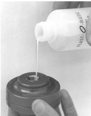
Plast-O-Matic gauge guards purchased with Plast-O-Matic gauges are factory filled. When purchased without a gauge, the installer must ensure that the upper gauge cavity and the gauge or instrument to be used must be solidly filled in order to accurately transmit the process line pressure or vacuum to the instrument. Air
