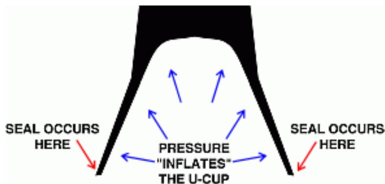
If a secondary or even a series of u-cups are used in the design, only the first one is pressurized, so friction is kept to a minimum. Secondary u-cups are used as backup seals in case the first u-cup fails.
