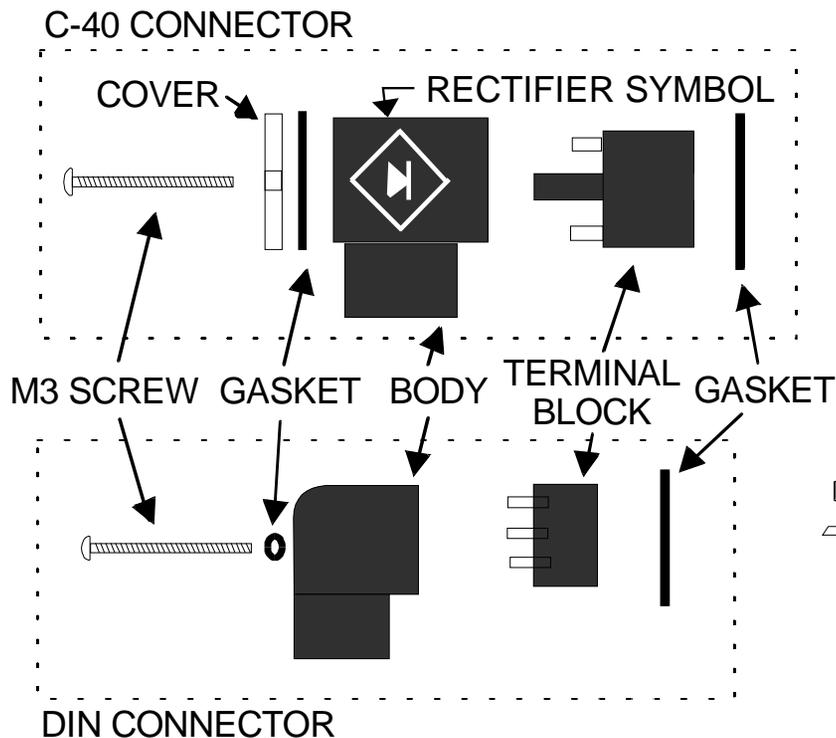
**WIRING** — Check voltage marking on coil before proceeding. The following is written for three wire power cord, adjust as needed for other wiring types. A small screwdriver is required. Wiring can be done before or after installing the coil or valve.
