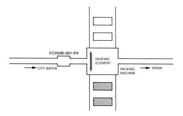
A major poultry processing company uses shrink wraps to seal its tray-packed chicken. The heat sealing element within the packing machine has been cooled directly via city water. This resulted not only in occasional damage to the heating
