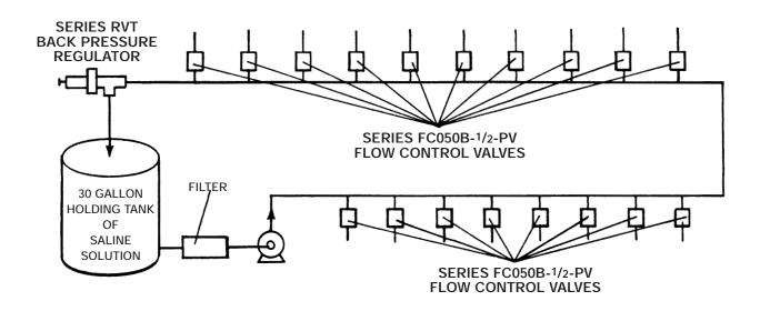
Following the manufacturing of contact lenses each lens must be individually washed with saline solution before packaged. Prior to incorporating the above products, each wash station had its own individual pumping system which was both expensive to operate and maintain. To resolve the problem the manufacturer redesigned the system using one pump for the entire process and installing
