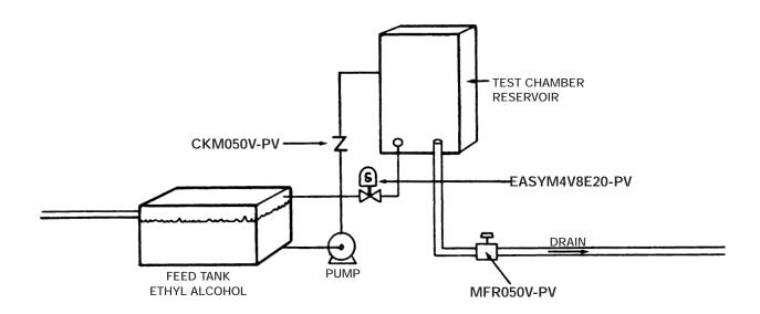
The above automated machine checks for faulty solder welds on finished printed circuit (PC) boards prior to installation. The PC boards are placed within the test chamber reservoir, then sealed. The ethyl alcohol is then feed into the chamber from the feed tank to a pre-determined level. Following the circuit weld testing the purity of the ethyl
