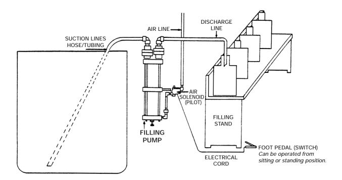
Contract filling/packaging company wanted an inexpensive yet accurate way to automate their manually-operated filling stations. By connecting a foot-operated pedal switch to a 4-way pilot air solenoid valve the operator was now capable of cycling the new Series VPA Metering Pump while
