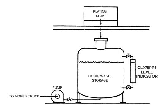
A circuit board manufacturer has a waste storage area in the company's basement. The area contains twelve (12) 6,000 gallon tanks for liquid waste storage of caustics, acid, water and various other chemicals used in etching PC boards. Waste liquids are gravity feed from the plating tanks on the first floor into the storage tanks in the
