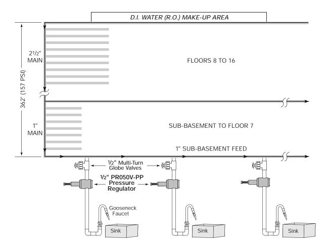
A world-renowned New York City hospital and research facility needed to protect its lab equipment and experiments from excessive pressure created by approximately 362 feet of head. The multi-turn globe pattern needle valves installed
