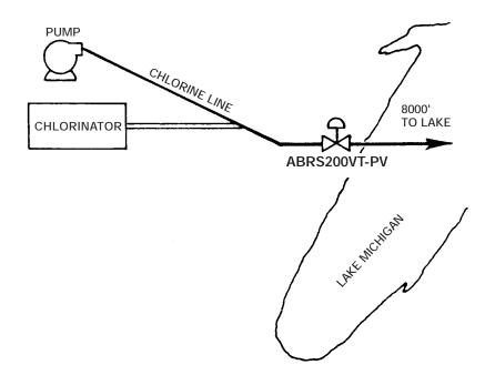
A water treatment plant on Lake Michigan required a 2" high flow, fail-safe pneumatic ball valve for their Zebra Mussel Containment System. The valve would control a chlorine feed line to the water treatment's 36" diameter, main intake crib located 8000 feet out in Lake Michigan. In addition to controlling the spread (growth) of Zebra Mussels at the mouth (crib) of the intake
