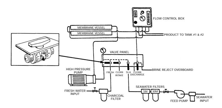
Manufacturer of desalinization equipment had been using brass ball valves to control flow sequences within R. O. systems. However, due to performance and difficulty of mounting (panel mounting-handles of ball valves had to be exposed and operated on face of valve panel)... the manufacturer selected the True Blue Valve that now provides him with non-corrosive components and with its molded mounting lugs - the simplest and most cost-effective method of panel mounting.
