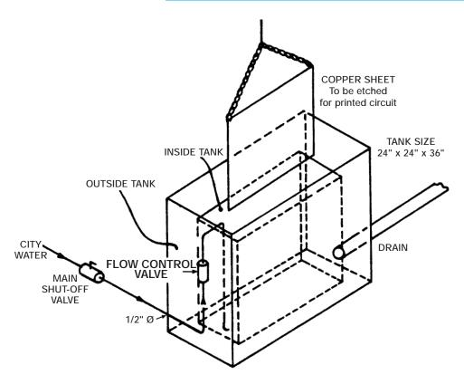
Following the etching of printed circuit (PC) boards, each one must be rinsed with water to remove excess copper. Prior to installing Series FC Flow Control Valves an excessive amount of city water was being consumed. To resolve this problem and conserve on water costs, customer evaluated
