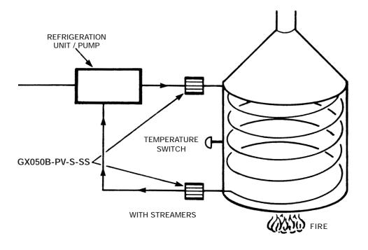
An English brewery incorporates an unique fermentation process in the manufacturing of their lager. By maintaining an elevated temperature throughout the fermentation process their yield increased dramatically. However, should the temperature exceed a specific point, the batch is lost. Running a coiled pipe inside the vessel enabled the brewer to introduce chilled water as a
