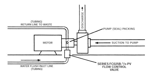
High performance centrifugal pumps which incorporate packing seals (glands) to isolate foreign material/build-up must be flushed or cleaned while operating. The flow and pressure through this packing must be constant to prevent them from causing damage. The installation of a Series FC Flow Control Valve provides the desired constant flow regardless of the fluctuating city water pressure feed.
