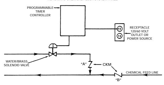
To assure that there is no residue remaining after each chemical addition, this chemical equipment manufacturer relies on two Series CKM Diaphragm Check Valves for two sequences. The "A" check valve is used to prevent chemical from attacking
