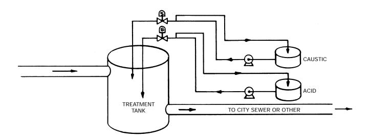
In typical industrial wastewater treatment systems, the effluent from the manufacturing area is transferred to the treatment tank where either a caustic base to raise pH or acid to lower pH, is injected to bring the pH into acceptable environmental levels. Direct acting solenoid valves are selected (Viton for acid, EPDM rolling
