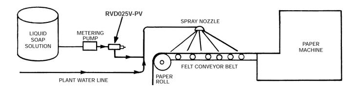
As paper stock leaves the machine it is wet and proceeds through a de-watering process. The conveyor is laid with felt to prevent the paper from becoming dirty. To keep the felt clean it is periodically sprayed with a liquid soap solution,
