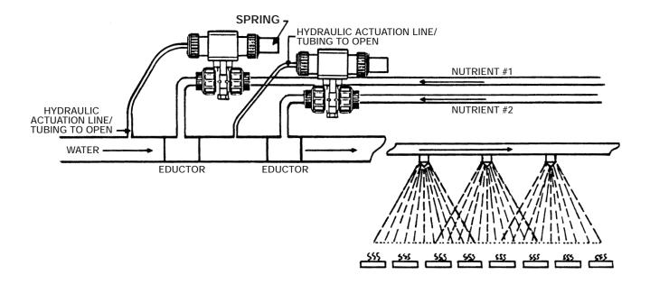
A major southern horticulturist needed a "Fail-Safe" method of automatic shutoff of liquid nutrients when his water pressure would drop below 40 PSI. This was necessary to prevent adding too much nutrient to the plants as a percentage of water. Since electricity was not readily available,
