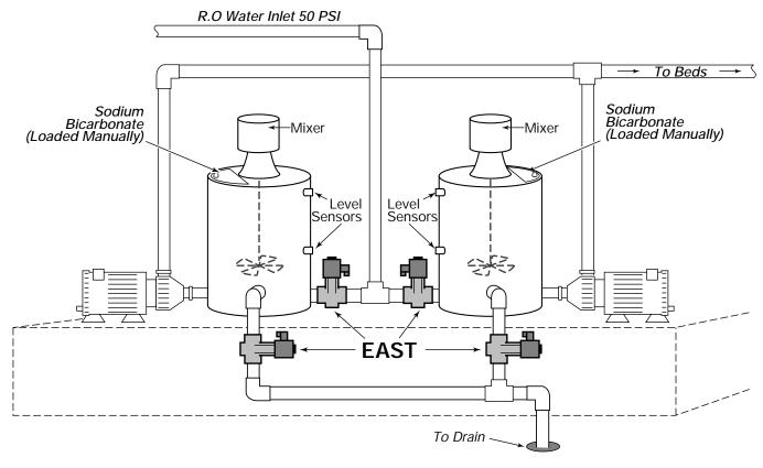
A worldwide dialysis equipment OEM required fail-safe, fast-acting valves for bicarbonate and R.O. water mixing. This "turn-key" system is designed for minimal maintenance as it is installed in dialysis clinics throughout the world.
