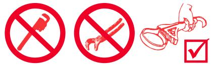
Proper care must be taken when threading a plastic valve into a piping system or failure of the valve body may result:
