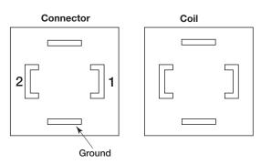
Terminals  $1\ \&\ 2$  are not polarity sensitive. Connector can be placed, wire facing up or down.
