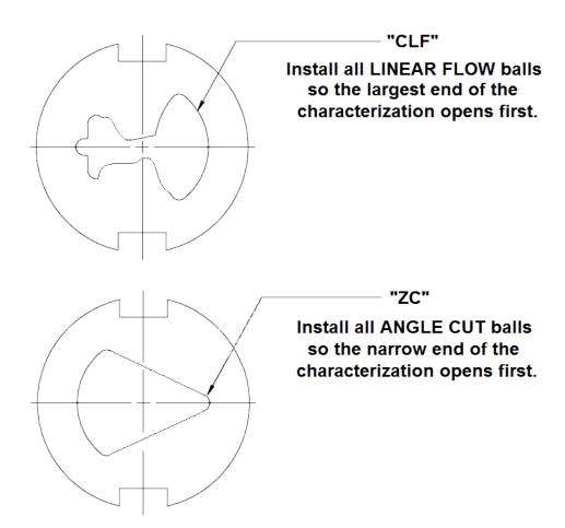
All Series ZC characterized balls must be oriented as shown so the appropriate end opens FIRST to achieve the intended flow performance. All angle cut balls must open narrow end first; all linear style-CLF must open larger end first.
